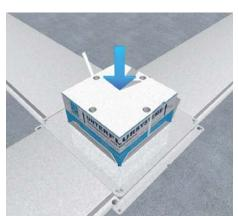
4 | Inserting the shuttering unit
